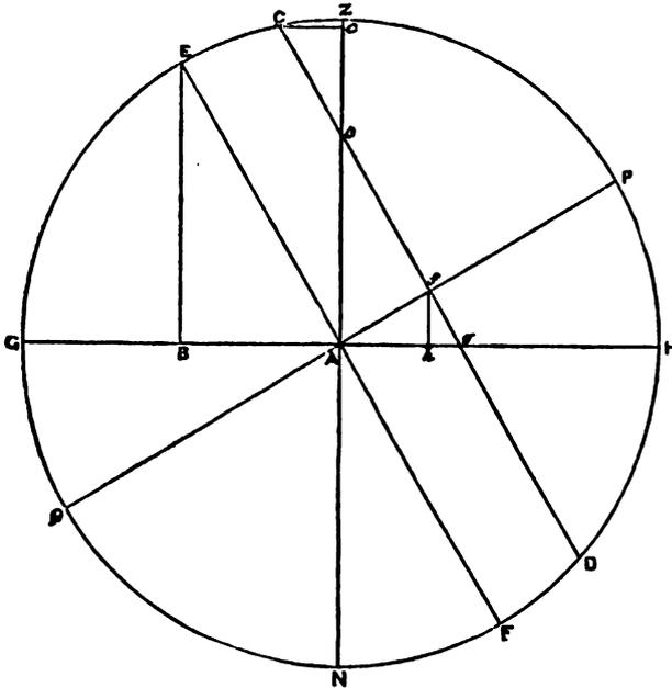
Let Z G N H be the meridian of the given place, G A H the diameter of the horizon, Z the Zenith, P and Q the north and south poles, E A F the diameter of the equinoctial, P A Q that of the six o'clock line, O f D that of one of the diurnal circles, and E B, f h the perpendiculars to G H. Then it is clear from this that
