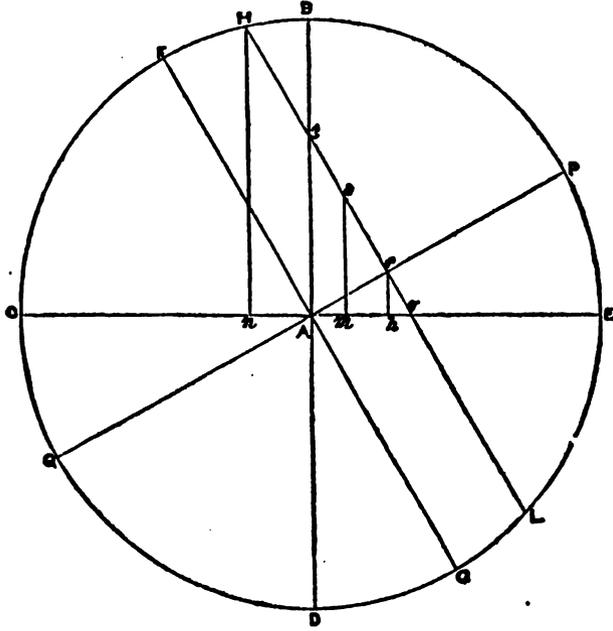
Let **B O D E** be meridian of the given place, **O A E** the diameter of the Horizon, **B** the Zenith, **P** and **Q** the north and south poles, **B A D** the diameter of the Prime Vertical, **F A G** that of the Equinoctial, **P A Q** that of the six o'clock line, **H f l** that of one of the diurnal circles, **s** the Sun's projected place in it and **f h**, **s m**, **H n** perpendiculars to **O E**. Then
