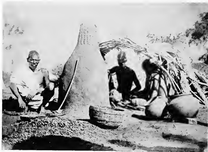
Fig. 24. Pariahs smelting small "blooms" of wrought iron, Salem district.
