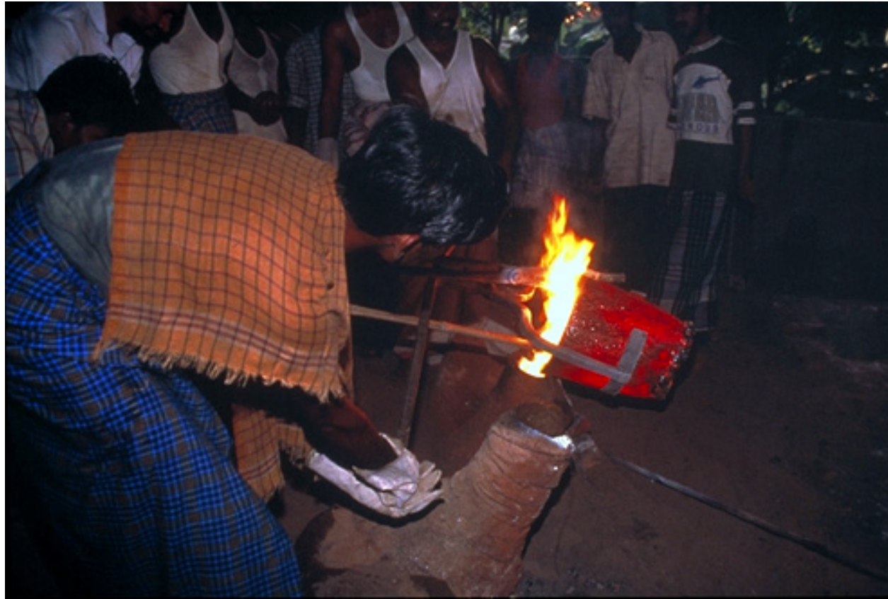
18. Lead and tin being poured into hollow clay mold.
