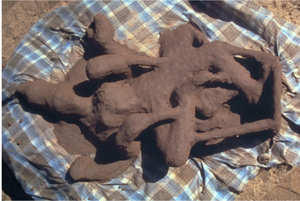
17. Completed wax model encased in several layers of clay.
