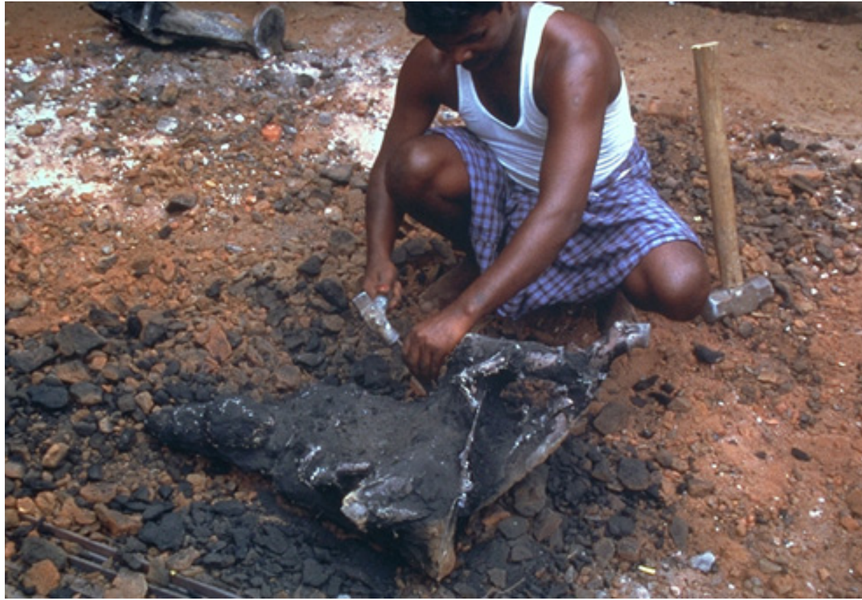
19. Breaking of clay mold to reveal bronze sculpture.
